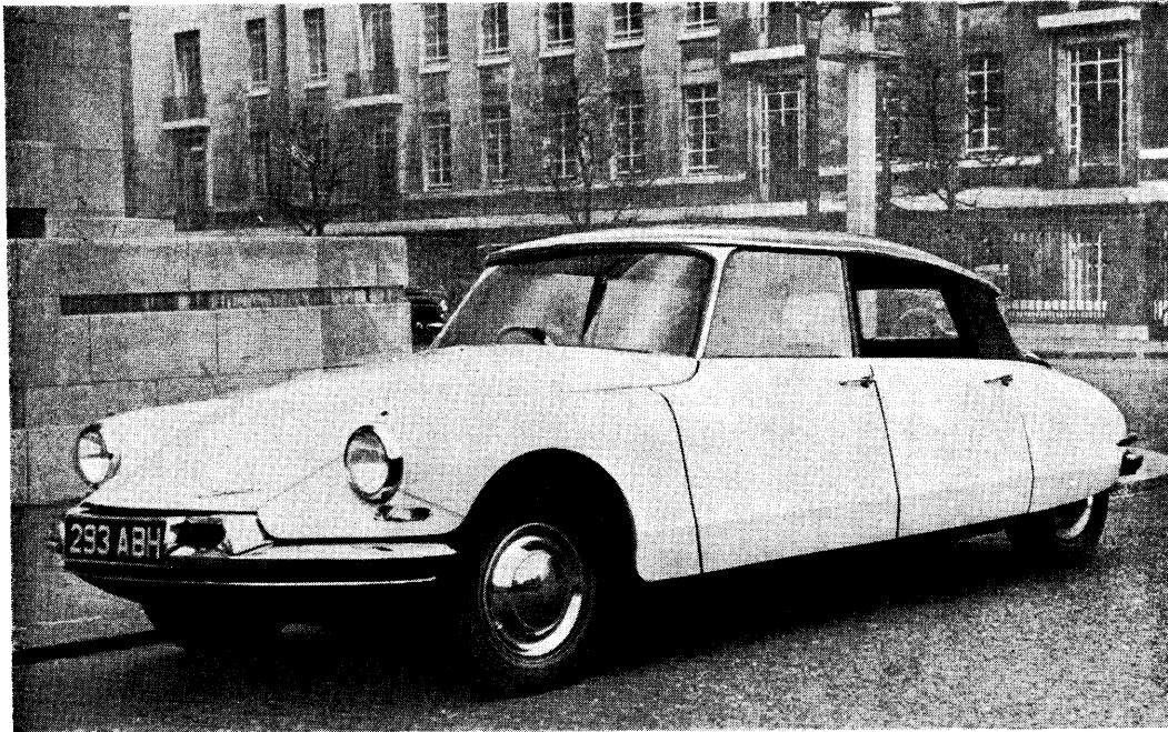
OUTLOOK from the DS19 is enhanced by the pronounced fall-away at the front, by the relatively high roof-line and by the extremely narrow front pillars. The front and rear wings may be detached after the removal of one nut.
