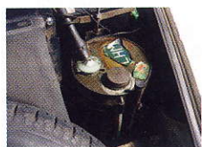
LHM fluid reservoir; one of the spheres it's pumped into
