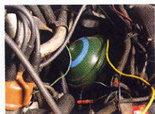
LHM fluid reservoir; one of the spheres it's pumped into
