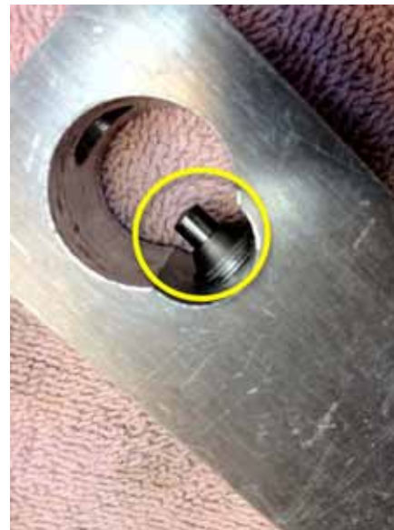
Photos #4 & 5: Revised Tool With Centering Guide
