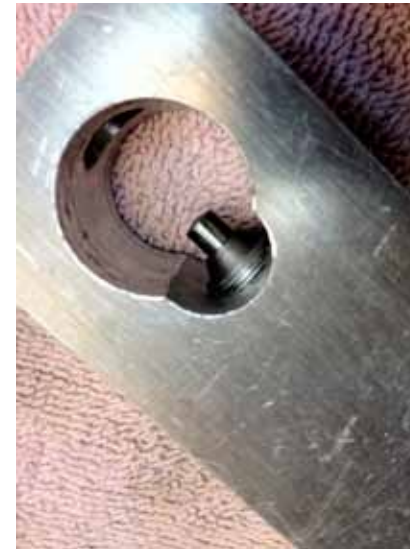
Photo #6: Revised Tool With Centering Guide
