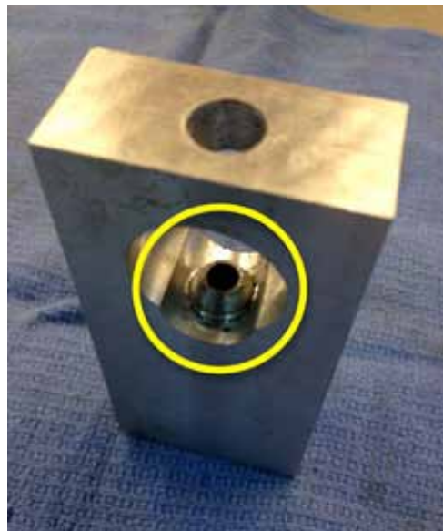
Photos #4 & 5: Revised Tool With Centering Guide
