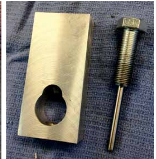
Photo #7: Revised Tool with Extraction Bolt Removed
