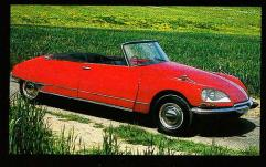
NOT CONTENT with building a car of perfect elegance, Chapron incorporated each evolution that the standard DS saloons underwent - larger engines, a facelifted front end (above) with cowled-in swivelling headlamps from 1967, and artificial fluid in the hydraulics to replace the rust-inducing hygroscopic castor-based oil in earlier systems. Each change improved the Décapotable immeasurably without dissolving its effortless finesse.
