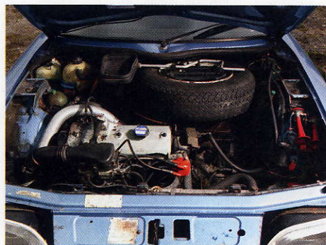
CX's variable-rate Diravi steering light but rock-solid on motorway; engine was transverse and canted 30° forward, which meant front discs went outboard
