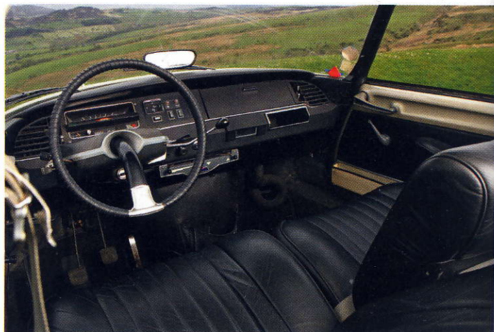
ID stands for Idée , or idea ; signature cornet de frites indicator; ID has a brake pedal, instead of the DS' famed 'mushroom' button; small hubcaps on most IDs
