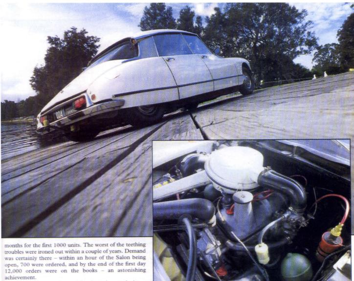
For those who were daunted by the DS's complexity, a simpler version, the ID, was announced a year later and although this shared basic principles with the DS, the hydraulics only worked the suspension.
